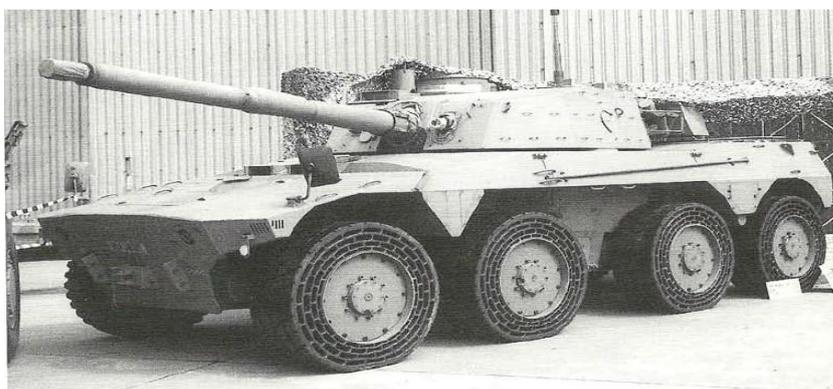
*The Rooikat with a South African designed set of airless tires that have been field tested and provide the operational performance required without compromising road speed.*
