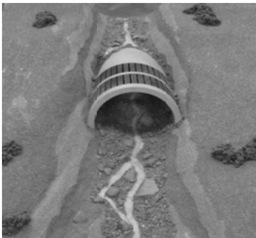
Fig. 5. General view of the through anti-mudflow Facilities of a springboard type (dummy)
